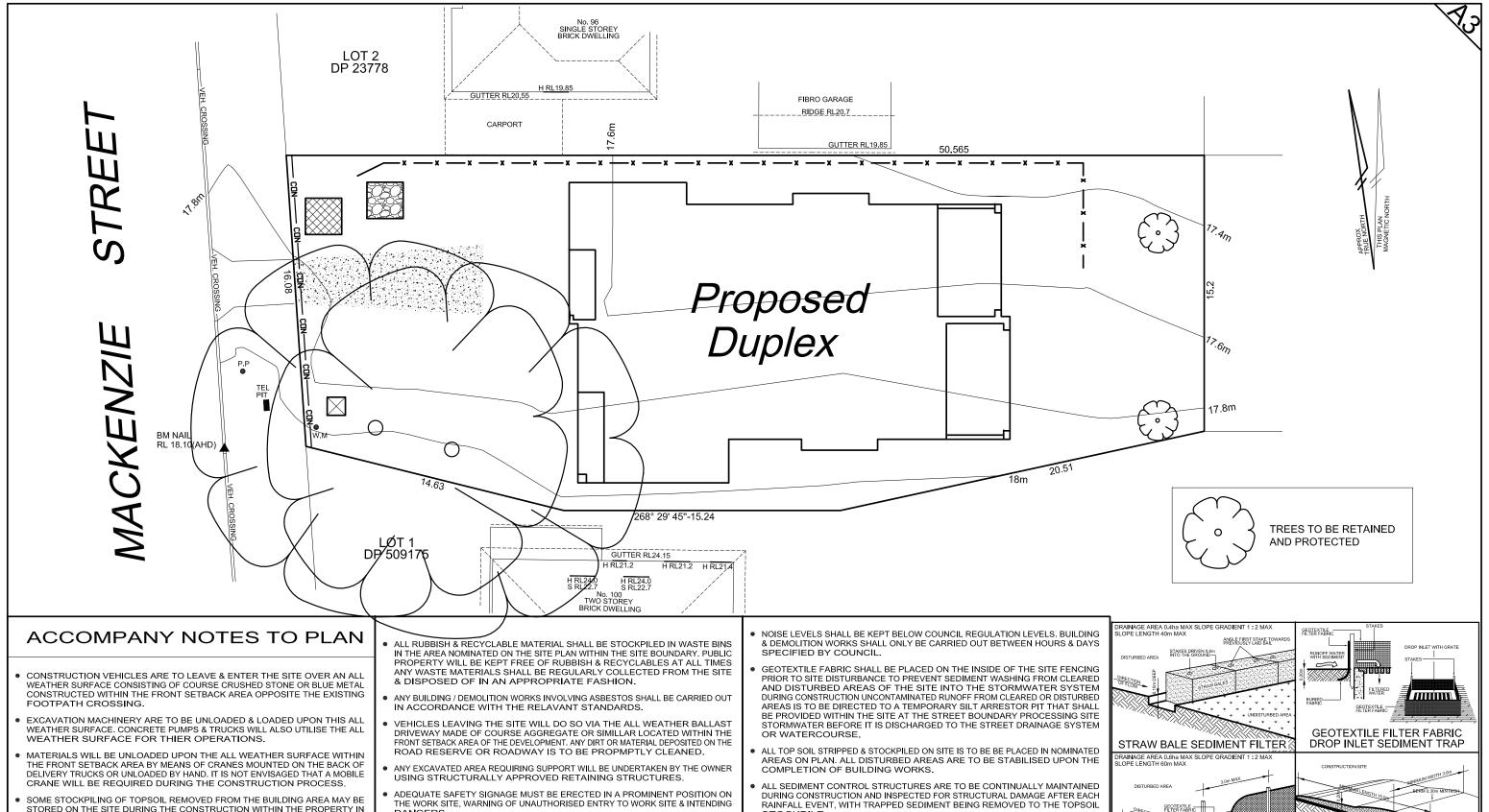
AN AREA ENCLOSED WITHIN THE SEDIMENT CONTROL FENCING. ALL EXCAVATED & CONSTRSUCTION MATERIALS, SHED, SKIP BINS, TEMPORARY WATER CLOSETS, SPOIL & EQUIPMENT, ETC SHALL BE KEPT WITHIN THE PROPERTY. NO VEHICLES OR MACHINES SHALL BE KEPT WITHIN THE PROPERTY.
